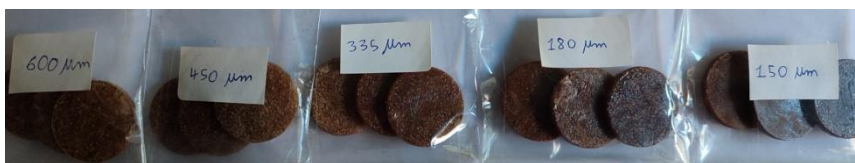
Figure 1. Biocomposites based on PLA, with 10% BSG of different particle size.
